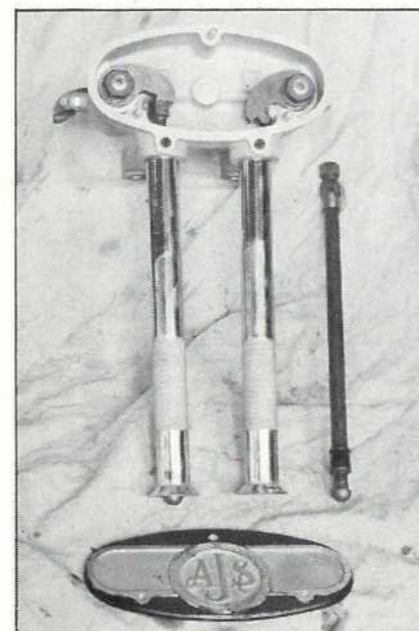
Knurled pushrod tubes are secured by grub screws; this early Thirties valve gear is lubricated by grease gun.
